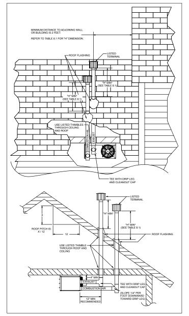
**Table 8.1 - Minimum Height from Roof to Lowest Discharge Opening**
