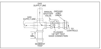
① Manual shut-off valve is in the "OFF" position when handle is perpendicular to pipe.
