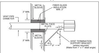
C9. When condensation may be a problem, the vent system shall not terminate over public walkways or over an area where condensate or vapor could create a nuisance or hazard or could be detrimental to the operation of regulators, relief openings, or other equipment.
