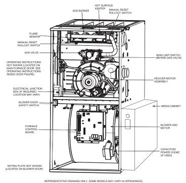
Fig. 1 – Furnace Components
