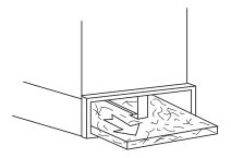
$\textbf{Fig. 23-Removal of Filter from Bottom Blower Cabinet} \ ^{A00228}$
