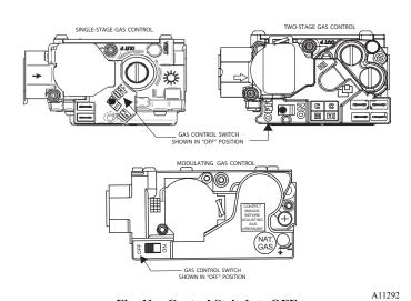
Fig. 11 - Control Switch to OFF
