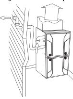
Fig. 3 – Interior Combustion - Air Pipe
