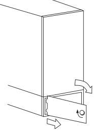
Fig. 21 – Removal of Filter Cabinet Door from Bottom Blower
