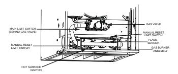
Fig. 27 - Gas Burner Assembly (Downflow)
