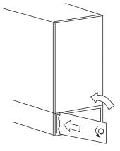
Fig. 25 – Replacement of Filter Cabinet Door to Bottom Blower
