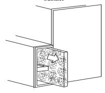
Fig. 22 – Removal of Filter from Side Blower Cabinet
