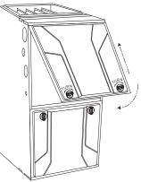
Fig. 13 – Furnace Door Replaced (Upflow Configuration)
