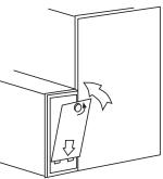
Fig. 24 – Replacement of Filter Cabinet Door to Side Blower
