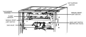
Fig. 26 – Gas Burner Assembly (Upflow)
